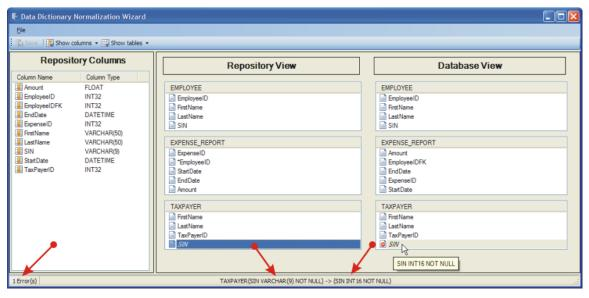
Table controls handle drag-and-drop. You can rename a column by dragging it from one table control to another or from the **Repository Columns**. Table controls also provide a context sensitive menu that enables you to:
